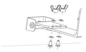
Adjust the required angle of the heater, and tighten the T-nut.
